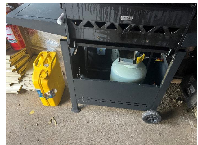
Photo 03. Class 2.1 Flammable Gases and Class 3 Flammable Liquids stored together in the Building D Mower Shed.
